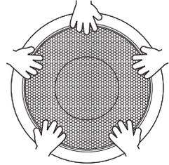
**Note:** Black butyl rubber tape is included for extra security in holding the grille in place. Cut four small pieces and space them equidistant around the groove in the baffle where the grille fits. The butyl rubber tape is quite sticky and it is not necessary to use an excessive amount.
