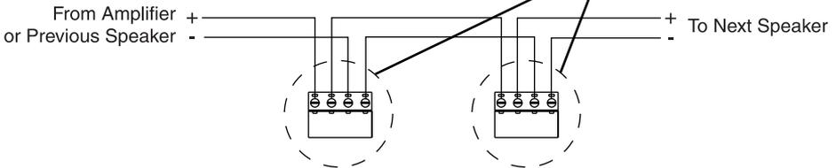
**Note:** When speakers are daisy-chained, disconnecting one speaker from the chain will disable all speakers further down the chain.
