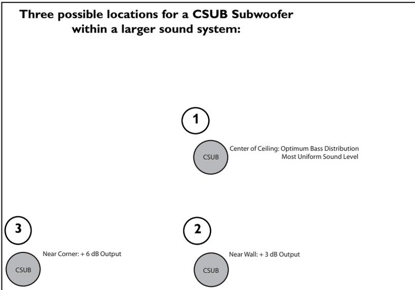
**Note:** The CSUB may be placed as close as 5" from a wall, provided care is taken to ensure that mounting clamps are properly extended (see *Installation* section). If mounting clamps cannot be properly extended, another location must be found.
