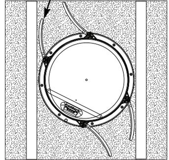
14-1/2 Inches between ceiling joists.
