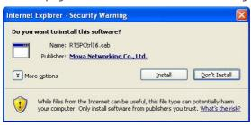
NOTE For Windows XP SP2 or above operating systems, the ActiveX Control component will be blocked for system security reasons. In this case, the VPort's security warning message window may not appear. Users should unlock the ActiveX control blocked function or disable the security configuration to enable the installation of the VPort's ActiveX Control component.
