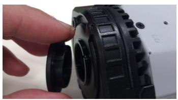
Step 2: Loosen the lens holder pressing screw with the L-type inner hexagon screw driver  $\,$
