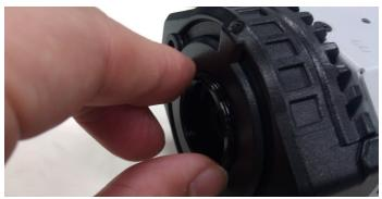
NOTE Make sure to loosen the screw affixing the lens holder in step 2 before trying to remove the lens holder. The lens holder may be too tight to loosen if screw is not loosened first
