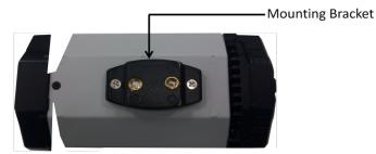
**NOTE** You will find the mounting bracket fastened at the bottom of the camera. You can remove and reposition the bracket to the top of the camera to meet your deployment requirements..
