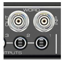
The received word clock signal can be distributed to other devices by using the word clock output. With this the usual T-adapter can be avoided, and the Fireface UCX operates as *Signal Refresher*. This kind of operation is highly recommended, because
