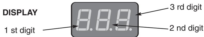
To gain access to setting menus press simultaneously on  $\ominus$  and  $\oplus$  keys on the Right. side during 5 seconds. (fig. 18). Menu 1 is displayed.
