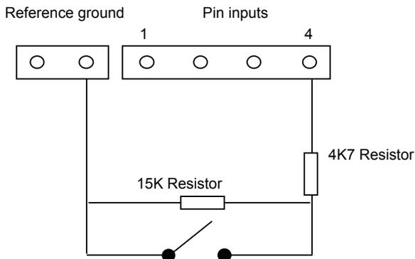
**Note:** For this feature to work correctly it is essential that the resistors are connected at the contact end of the loop and not the dialer end. The Monitoring Centre must also enable this facility on the dialer.
