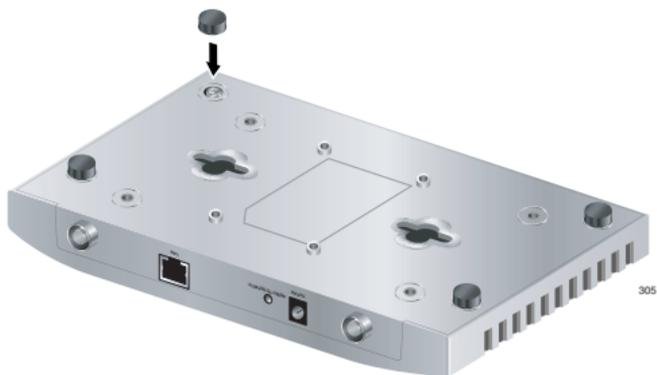
Figure 5. Attaching the Rubber Feet
