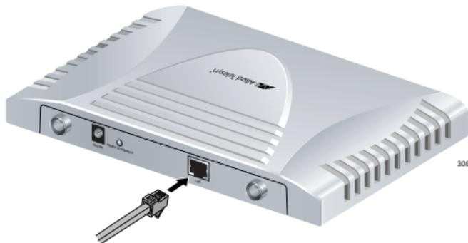
Figure 8. Attaching the LAN Cable
