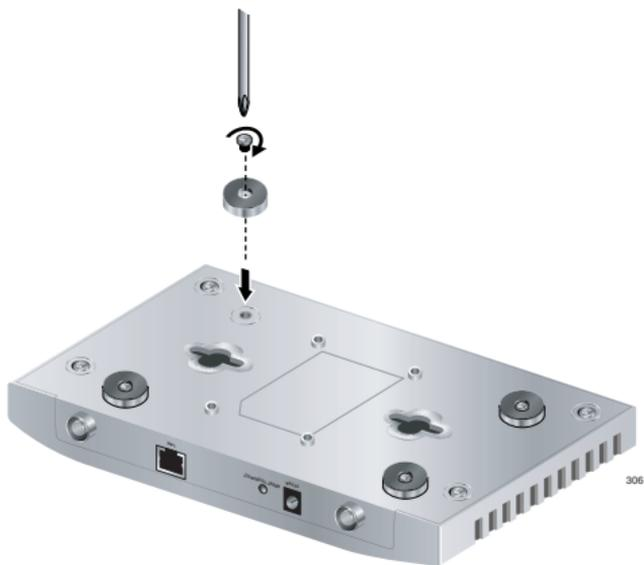
Figure 7. Attaching the Magnets
