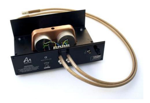
Once located, connect the AN-S9 between your turntable and phonostage input. Connect your tonearm / turntable output cables to the input sockets on the AN-S9, and the output cables of the AN-S9 to your MM phonostage input.
