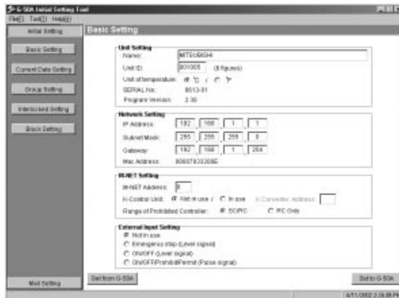
Figure 15-1 Example of screen for initial setting tool
