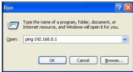
Running a ping test to the LAN from the computer
