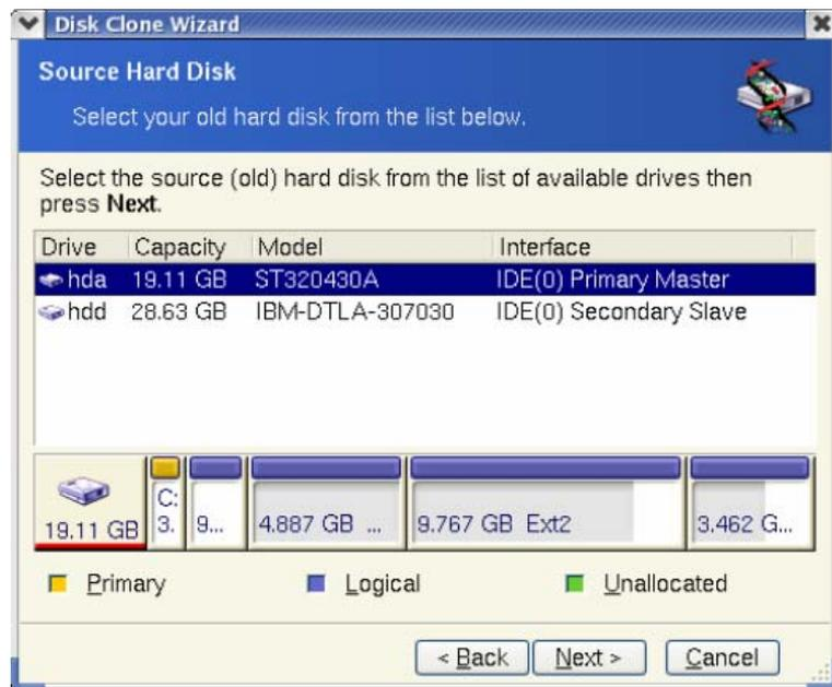
You can determine the source and destination using the information provided in this window (disk number, capacity, label, partition and file system information).
