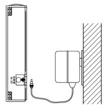
Insert 2 AA batteries and connect the included AC adapter (AC120V, 60Hz-DC5.0V, 100mA).
