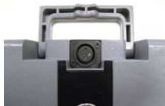
Electric Bikes with Rack Mounted Battery (RMB) Packs - Lift the battery pack handle to expose the charger port and attach charger.
