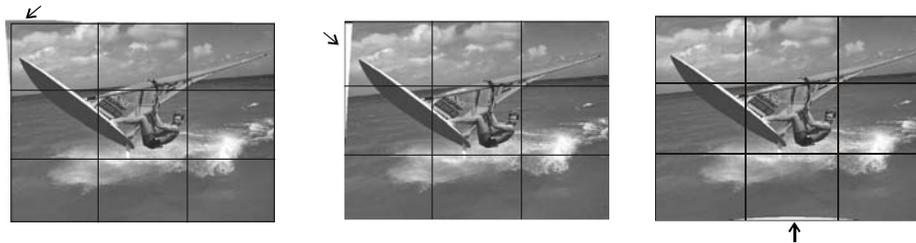
You can also use the mirror to correct slight misalignments between projected images where the edges align properly with the screens, but adjoining images do not line up correctly.
