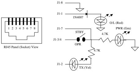
Figure 1: ARI-500 Interface Unit Schematic
