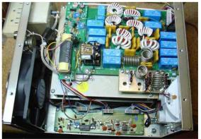
Photo B: New relay-switched low pass filter board permits remote band switching.
