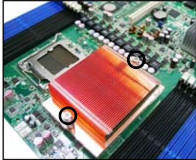
2. Secure the heatsink with two screws.
