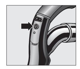
The first time the vacuum cleaner is switched on, the highest power setting will be selected automatically.
