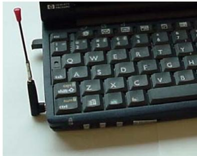
*Figure 5-1: Proper positioning of the AirCard antenna*
