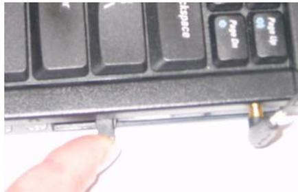
*Figure 5-2: Ejecting the AirCard from its slot*
