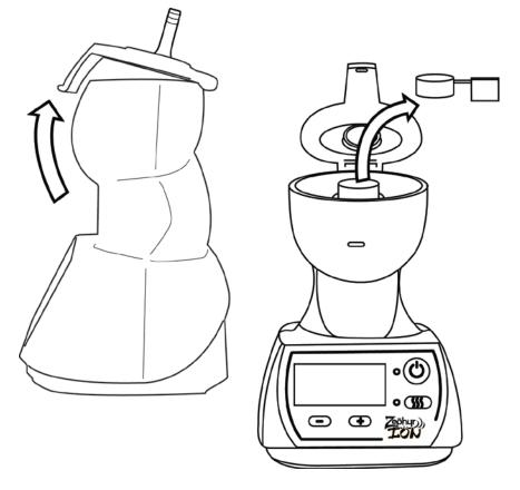
To prepare your vaporizable material, you should first grind the material and then place it loosely in the basket. You can fill the basket as little or as much as you like. Typically, we recommend filling the basket between 1/3 and 1/2 full. The goal when grinding your vaporizable material is to create as much surface area as possible for the hot air to flow over, so grind finely to maximize surface area and vapor. Never stuff or pack material into the basket.
