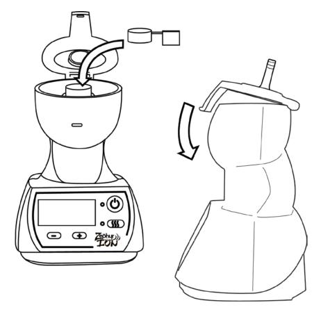
Once the desired temperature has been reached (the Ion's LCD screen turns green), open the lid of the Ion and place the basket in the basket holder. Make sure that it is sitting flat before attempting to close the lid. The lid will close easily when the basket is seated correctly. Forcing the lid against an improperly positioned basket could damage the unit.
