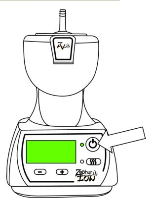
Turn the unit on by pressing the 'Power' button once. The power LED will change to green to show that the heating element is on. The LCD screen will remain red and the desired temperature will flash as the unit is heating up. Once the unit has reached the desired temperature the LCD screen will turn green.
