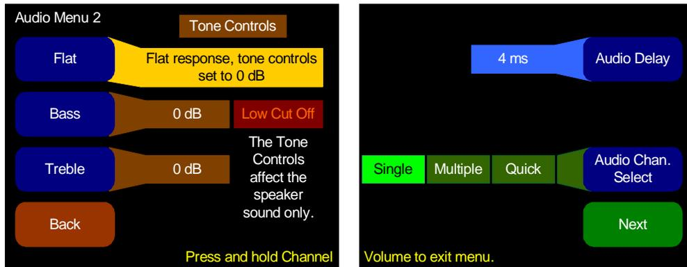
Pressing the **Flat** button brightens the **Flat** setting and darkens the **Bass** and **Treble** settings to brown, and produces a flat response. This is the default setting. However, the **Bass** and **Treble** settings are retained so you can recall them the the next time you press the **Flat** button, the **Bass** button, or the **Treble** button.
