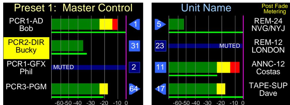
You can mix and monitor any or all of the eight metered channels in three different methods: quick selection, single channel selection, or multiple channel selection.
