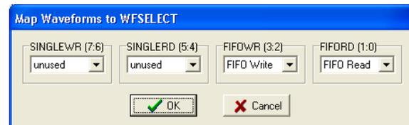
Make sure that the FIFO Write waveform is mapped to FIFOWR and the FIFO Read waveform is mapped to FIFORD. This ensures that when GPIF FIFO Write operation is launched, the FIFO Write waveform is executed and when a GPIF FIFO Read operation is launched, the FIFO Read waveform is executed. The mapping of bit fields is identical to the bit fields in the GPIFWSELECT register. The waveforms are already mapped appropriately; click **OK**.
