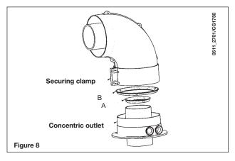
If the flue outlet is placed outside, the flue-air ducting must protrude at least 18mm out of the wall to allow alluminium weathering tile to be fitted and sealed to avoid water leakages. Ensure a minimum downward slope of 1 cm towards the outside per each metre of duct length.
