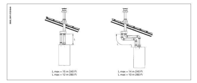
**Important:** if fitting a single exhaust flue duct, ensure it is adequately insulated (e.g.: with glass wool) wherever the duct passes through building walls.
