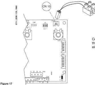
Connect the cable, supplied as an accessory together with the external probe, to the **CN10** connector of the boiler electronic board, as illustrated in figure 17. When the external probe is connected, the heating circuit temperature control device (2 - figure 1), regulates the dispersal coefficient Kt (Figure 18).
