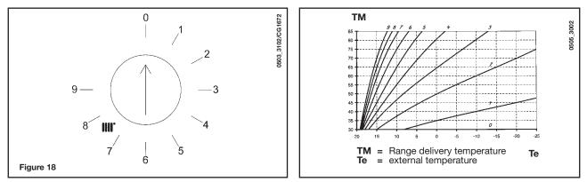
**IMPORTANT:** the **TM** delivery temperature value depends on the position of the jumper or the switch T.RISC. (section 23). The maximum possible temperature setting is 85 or 45°C.
