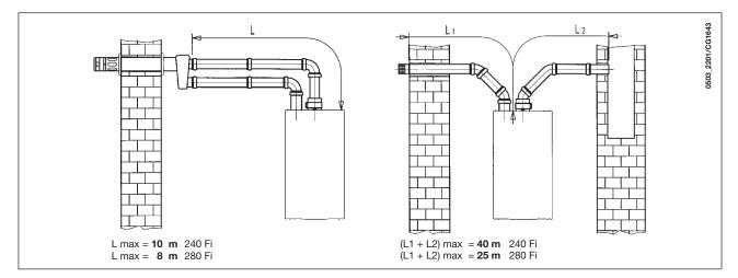
**NB:** For C52 types, terminals for combustion air suction and combustion product extraction must never be fitted on opposite walls of the building.
