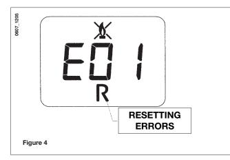
To RESET the gas boiler, turn selector (Figure 2) to "R" for at least 2 seconds. If the fault persists, call an authorised service centre.
