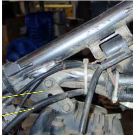
Right Side Cable Routing
