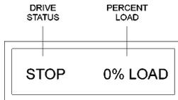
Pressing the ENTER key again will change the display from the % LOAD indication to the VAC (motor voltage) indication:
