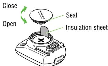
**CAUTION !** When closing the battery cover, be careful not to pinch the seal. Doing so may adversely affect the splash-proofing seal and result in a malfunction.
