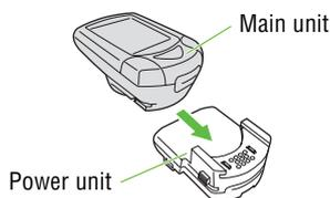
**NOTE:** Be sure to attach the main unit to the power unit. If formatting or a restart is carried out using the main unit only, unnecessary data may remain in the power unit, resulting in a malfunction.
