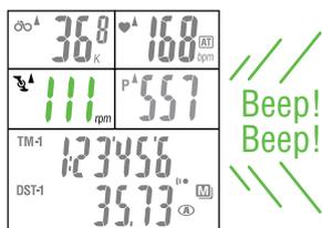
**NOTE:** When both the heart rate and the cadence are turned on and go out of the respective zones, the heart rate and cadence values flash.
