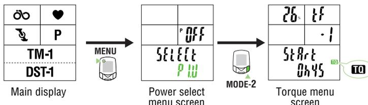
**NOTE:** Before carrying out torque measurement, set the data storage option to ON. The torque measurement data are recorded to a data file in the same way as data are stored. Therefore, the torque measurement menu is not displayed when the data storage option is OFF.
