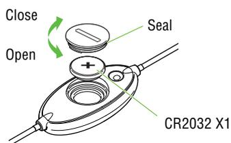
transmitter. Replace used battery with a new lithium battery (CR2032). Place battery with the + sign upwards as shown in the illustration, and firmly close the battery cover.
