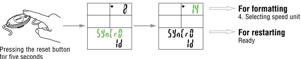
**NOTE:** If the HR sensor is placed too close to the main unit (within 20 cm), the main unit cannot receive the ID signal. If an ID check failed, change the distance, and reset the heart rate sensor. If "E" appears on Display-2, or a HR sensor ID check failed even at a proper distance, the batteries may be dead. Replace the batteries of the heart rate sensor in the procedure shown on page 65, and format (restart) the computer again.
