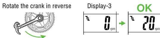
**NOTE:** If all numbers do not appear, this means that the magnet is positioned incorrectly in relation to the sensor. Check the position of the magnet, referring to the accompanying “Installing the unit on your bicycle”.
