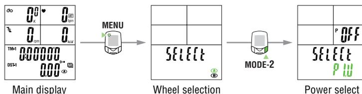
2. Press the START/STOP/ENTER button and then the MODE-1 or MODE-2 button to set the Power select option to ON. When the START/STOP/ENTER button is pressed again, calibration starts and checks whether or not the unit is connected to the power sensor correctly. After calibration has been completed, the software of the main unit is available to the power unit.
