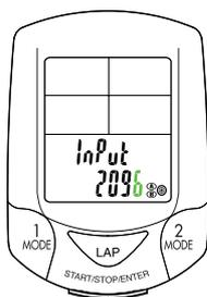
Enter the circumference of the tire of your bicycle in mm. 2096 mm (700 x 23 C) is preset as the initial value. To change the value, use the MODE-2 button to increase the value, and use the MODE-1 button to shift the digit. Pressing the START/STOP/ENTER button and this is the last step in the initial set-up.
