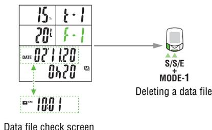
**NOTE:** When a data file is deleted, the numbering sequence of the remaining files is advanced.
