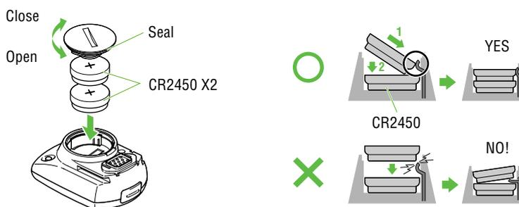
Replace the old batteries with new lithium batteries (CR2450). Place two batteries with the + sign up, as shown in the illustration, and firmly close the battery cover.
