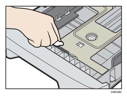
5. Wipe the rubber part of the roller with a soft damp cloth. After that, wipe it with a dry cloth to remove moisture.
