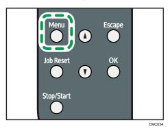
2. Press the [▲] or [▼] key to display [Host Interface], and then press the [OK] key.
