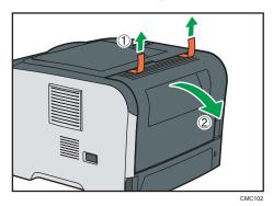
5. Pull out the tape, and then remove the protective materials.
