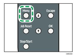
2. Press the [▲] or [▼] key to display [Paper Input], and then press the [OK] key.
