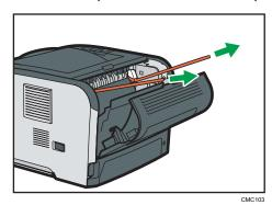
The actual printer may come with protective materials attached in different positions. Make sure to check the printer's exterior for all protective materials, and remove them completely.
