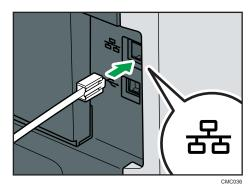
2. Connect the other end of the cable to the printer's network, such as a hub.
