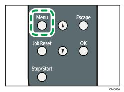
2. Press the [▲] or [▼] key to display [Host Interface], and then press the [OK] key.
