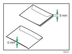
• If the curl is severe, flatten out the envelopes using your fingers, as shown in the illustration below.
