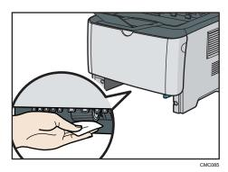
6. Reload the removed paper into the tray, and then push the tray carefully into the printer until it clicks into place.
