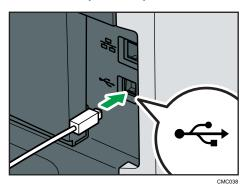
2. Connect the opposite end's flat connector to devices such as your computer's USB interface.
