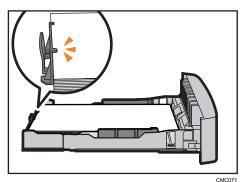
6. Carefully push tray 2 straight into the printer.
