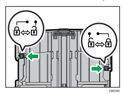
5. Pinch the clip on the side paper guide, and then slide it to match the standard size.
