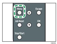
2. Press the [▲] or [▼] key to display [Paper Input], and then press the [OK] key.
