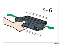
10. Slide the print cartridge in horizontally. When the cartridge can go no further, raise it slightly and push it fully in. Then push down on the cartridge until it clicks into place.
