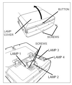
Figure 1. Lamp Cover and Lamp Assembly Removal
