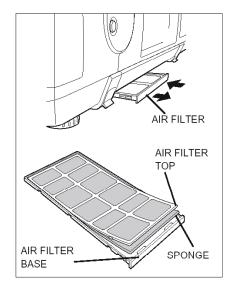
Figure 4. Air Filter Removal
