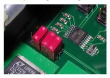
For dual wire format remove the 1st jumper:
