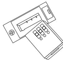
**Figure 3-3 Battery and Battery Charging Cup**
