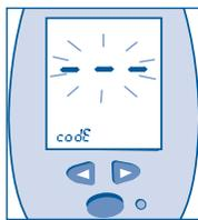
**IMPORTANT:** If the code number on the display does not match the code number on the test strip vial, the test results may not be accurate.
