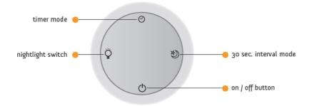
immediately runs the machine on / off button timer mode
