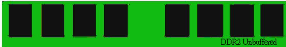
Before installing your memory sticks, please ensure that the memory sticks you have are compatible with the SW44X. The SW44X will only support DDR2-667/533/400 modules. Please study the table below for memory module specification of the SW44X.
