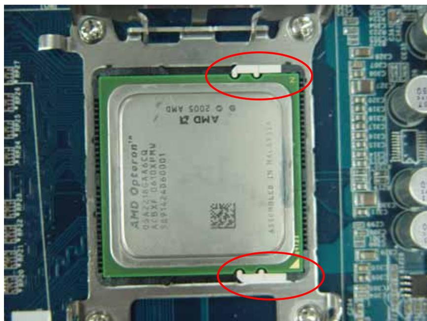
5. Close the metal cover and return the lever into its original locked position.
