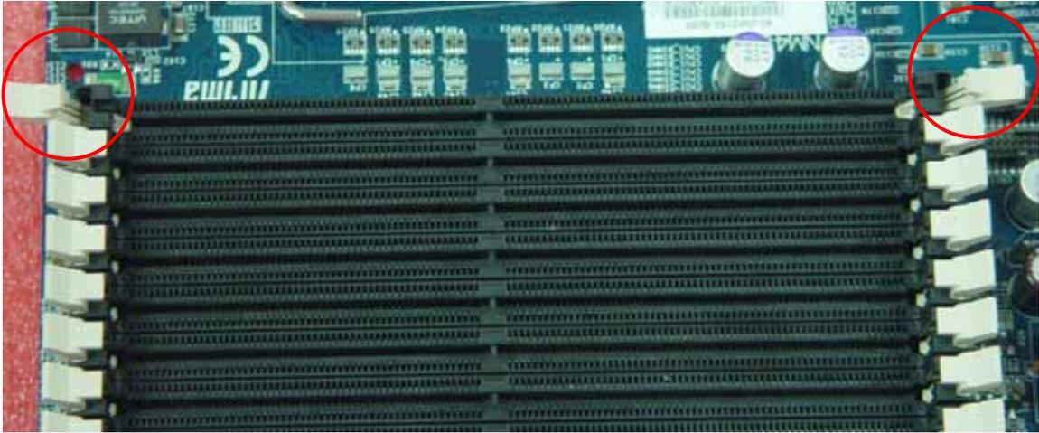
2. Line up the memory with socket. Make sure the gap fits into the socket.
