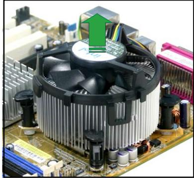
5. Rotate each fastener clockwise to reset the orientation.
