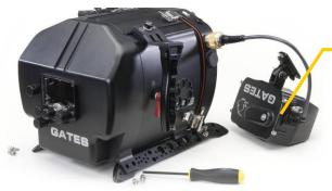
Note: If you are opening the shell after a dive, secure the monitor to the top of the front shell or set off to the side of the housing.
