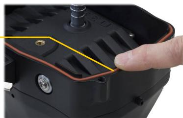
**Close the monitor shell.** Mate the rear shell to the housing. Insert and tighten the 4 screws until snug. Tighten until there is no visible gap between shells. A good indicator is when the orange o-ring is no longer visible.
