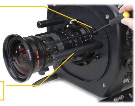
Thread the Guide Bar into the front shell and tighten by hand.
