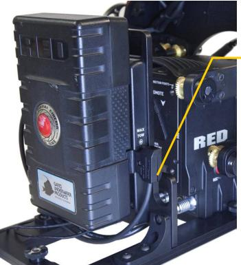
Install the Power connector here, on the side of the V-Lock battery mount.
