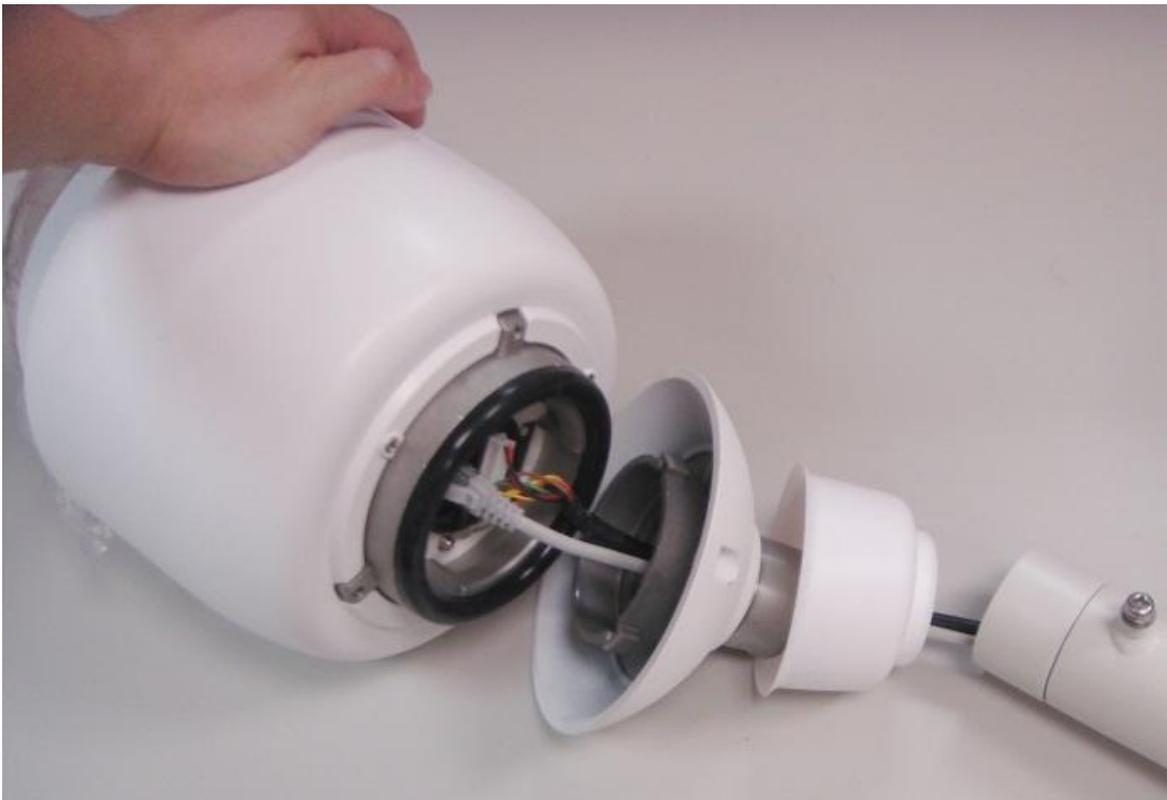
There are three locking areas on the mount kit. Put it on top of the speed dome, then rotate it into position.
