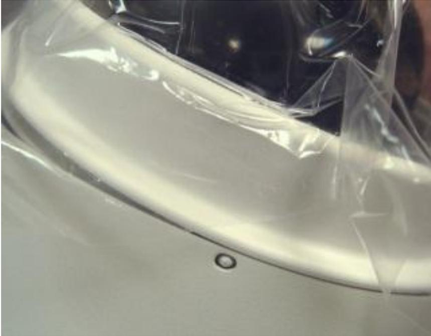
Secondly, there are two metal screws at the sides of the dome cover. Use a flat headed screwdriver and unscrew them. Unscrewing will extend them outwards, securing the dome cover.
