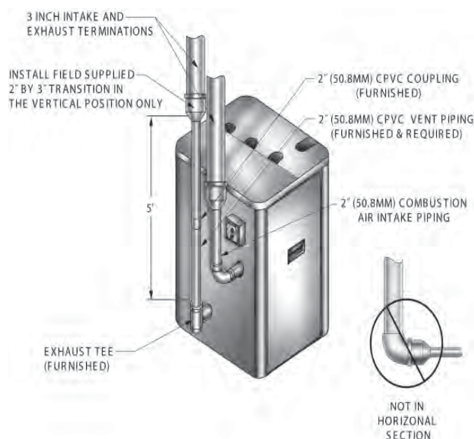
Figure 11 - Combustion Air & Vent Piping
