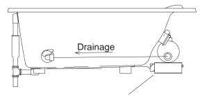
Shim if necessary, using 5" x 7" (minimum) plywood
