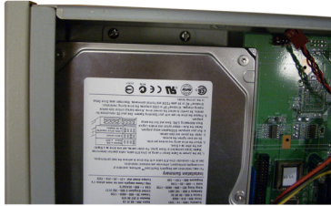
Figure 2.3: Install the standard drive bay
