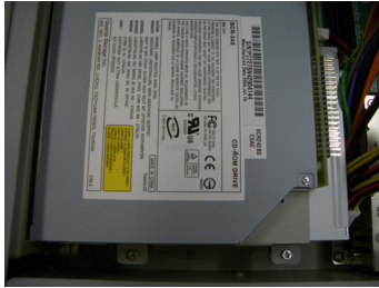
Figure 2.5: Install the standard drive bay
