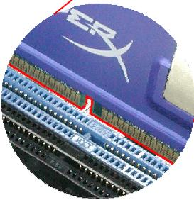
**Note:** The tabs of the DIMM slot will clip to hold the DIMM in place when the DIMM touches the slot's bottom.
