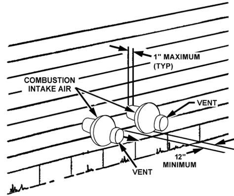
Figure 30: CONCENTRIC VENT TERMINATIONS FOR HORIZONTAL DIRECT VENTING
