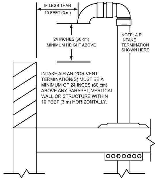
**VERTICAL TERMINATION(S) FLAT ROOF CLEARANCE**
