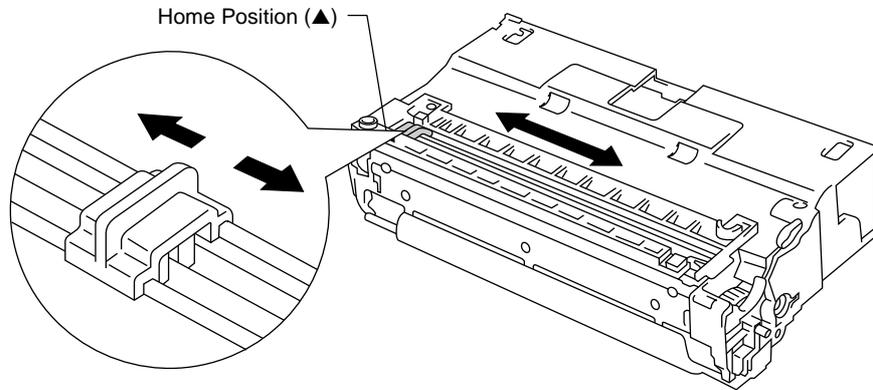
**Fig. 5-18 Cleaning the Primary Corona Wire**
