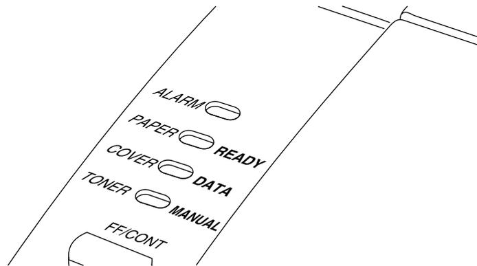
Fig. 3-1 Lamps on Control Panel
