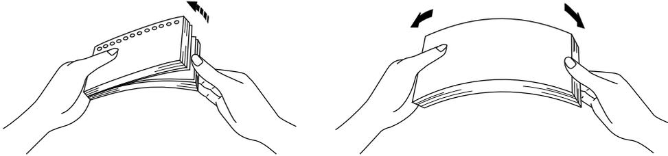
**Fig. 2-1 Fan the Paper and Straighten the Paper**
