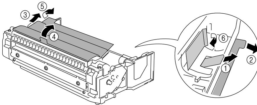
Fig. 5-12 Removing the Protective Parts
