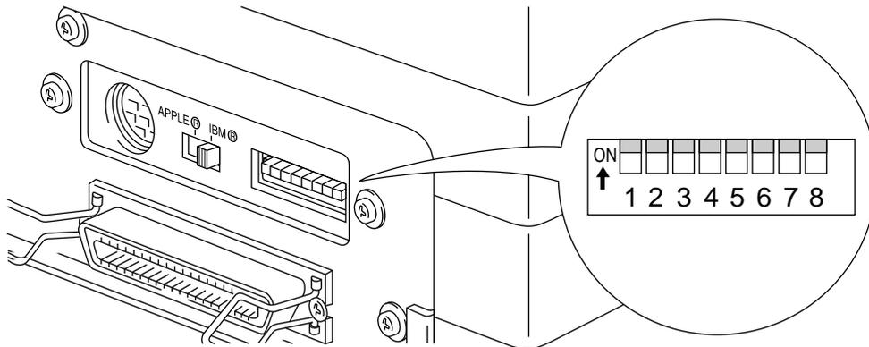
Fig. 4-3 Setting the Serial Interface Parameters
