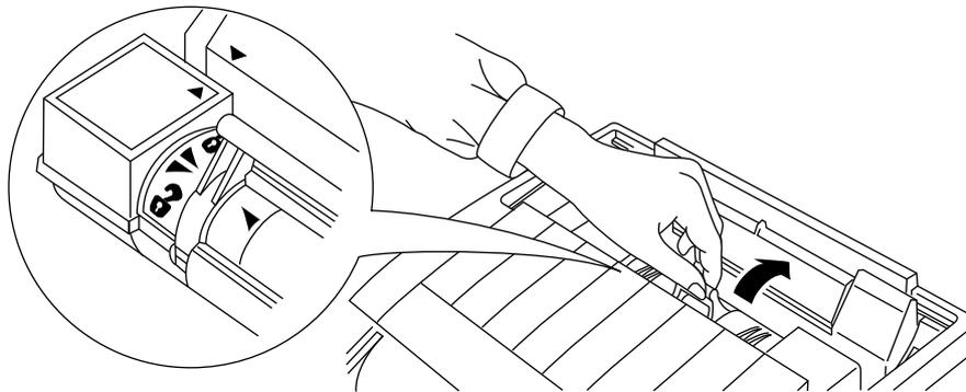
**Fig. 5-3 Closing the Shutter of the Toner Cartridge**
