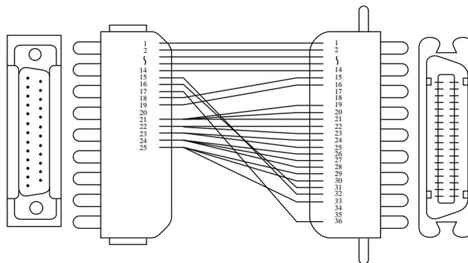
Fig. A-1 Parallel interface cable
