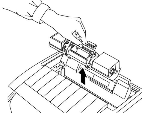
Fig. 5-4 Removing the Old Toner Cartridge
