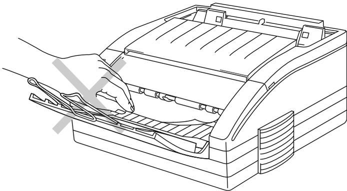
Fig. 6-2 Paper Jam at the Paper Output Tray
