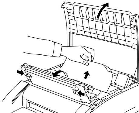
**Fig. 6-4 Paper Jam under the Drum Cover**
