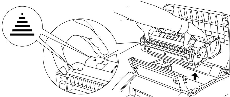
**Fig. 5-19 Removing the Drum Unit Assembly**
