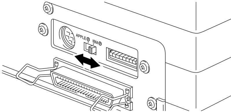
**Fig. 4-2 Selecting the RS-422A (Apple) or RS-232C (IBM) Serial Interface**
