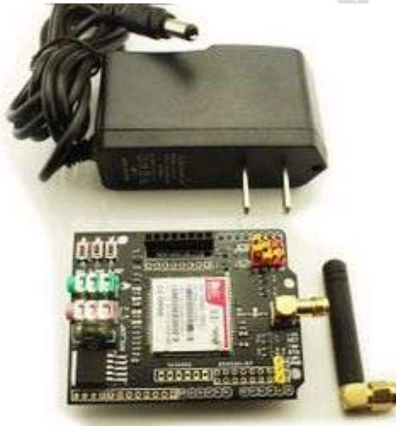
This GPRS Shield is compatible with all boards which have the same form factor (and pinout) as a standard Arduino Board. **GPRS module** delivers GSM/GPRS 850/900/1800/1900MHz performance for voice, SMS, Data, and Fax in a small form factor.
