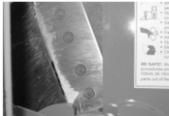
WORN & CHIPPED KNIFE EDGE
