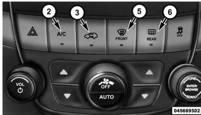
Automatic Temperature Controls — Hard-Keys
