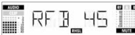
Example 3: Antenna B was active for 45% of the test period.
