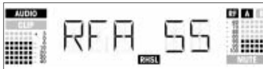
Example 2: Antenna A was active for 55% of the test period.
