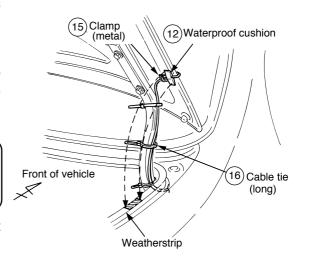
Route the GPS antenna cable to the main unit while securing it with harness fixing tape.
