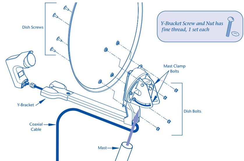
2. Assemble new 51 cm Multi-Satellite Dish by attaching mount plate bracket to the back of the satellite dish with supplied screws and bolts. Attach Y-adapter bracket to dish support arm using Y-bracket screw and nut.
