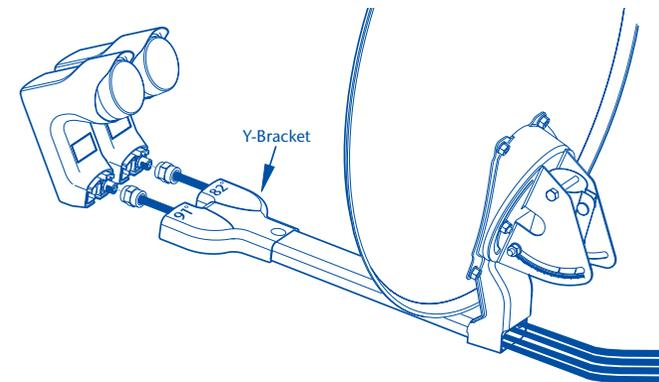
4. At the back of the dish assembly, thread the other two coaxial cables through the inside of the satellite dish arm until the cables protrude through the opening of the Y-adapter labeled 91°. Label these cables at 91° to help identify them when connecting them later.
