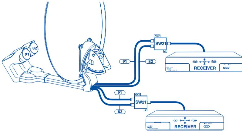
8. Connect the cable(s) that will go inside the home to the output(s) of each 2:1 multi-switch
