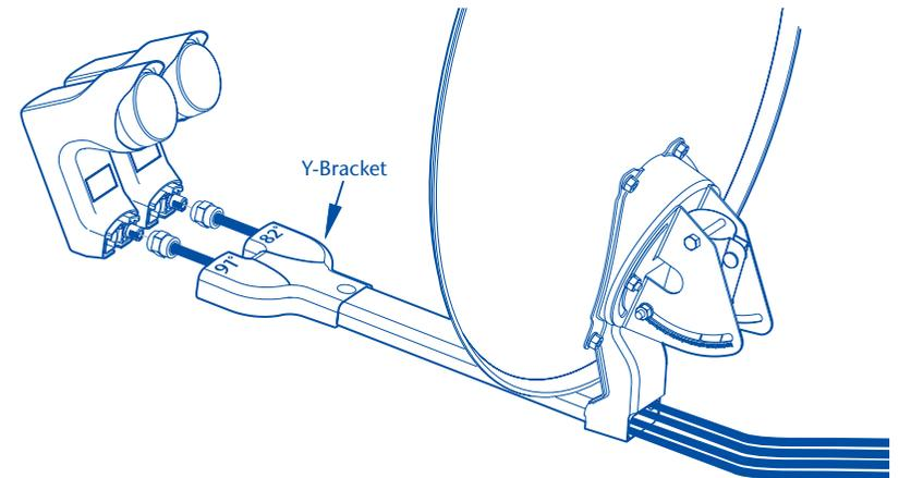
3. Connect end of coaxial cable to the new LNBF that was packed in your Upgrade Kit. Attach the LNBF to the Y-adapter and secure it with the LNBF screw and bolt.
