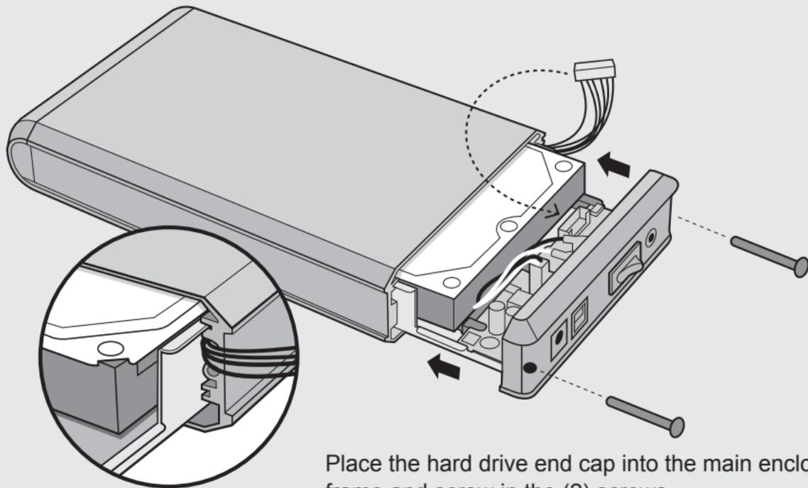
Place the hard drive end cap into the main enclosure frame and screw in the (2) screws.
