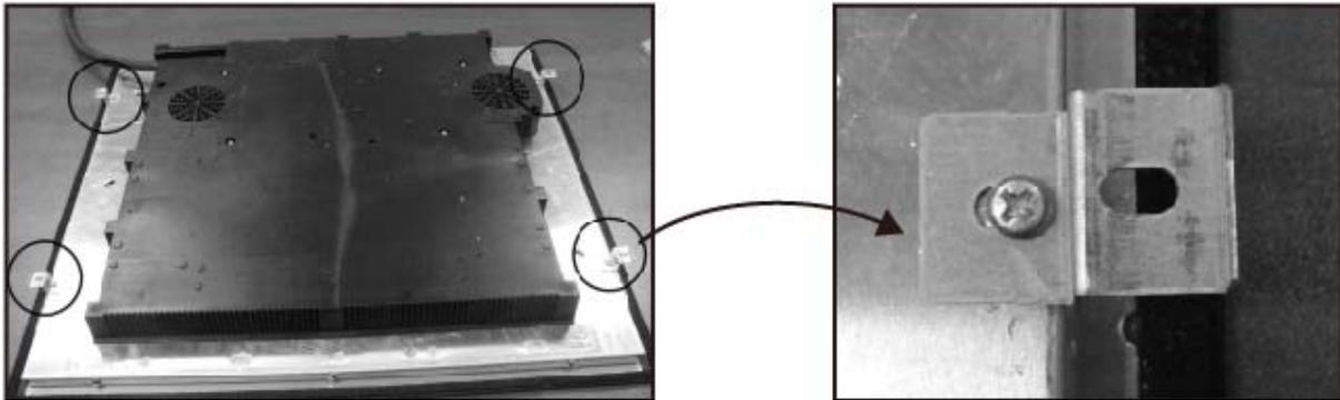
You should place the bracket on the underneath of the hob, in a position that is appropriate for the aperture that you have cut out. Using the screws provided, fix the bracket to the hob. These screws **MUST** be securely tightened.
