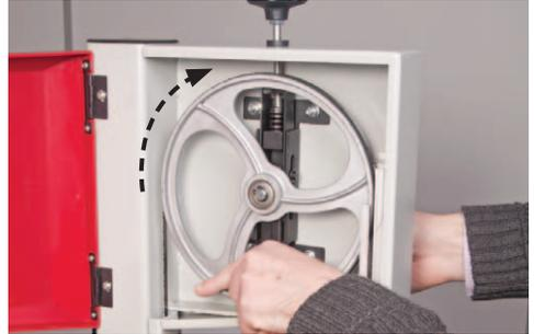
upper saw wheel by hand. Loosen the upper blade guide clamp and set the upper blade guide assembly so that the top of the blade guide is level with the centre of the top drive wheel, see fig 33. Re-tighten the clamp.
