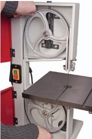
lower blade guides, see fig 31. Apply some tension to the blade. Turn the top wheel by hand to ensure the blade will not skip off the wheels and the blade is travelling in the blade guides, see fig 32. Apply a little more tension and check by once again spinning the
