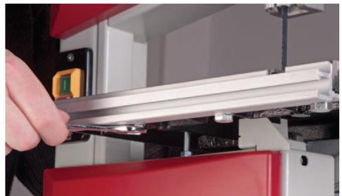
**Step 3** Locate the fence assembly (D). Lower the fence over the table until the clamping lever assembly slots into the fence rail's "T" slot. **NOTE: Make sure the clamping hook to the rear of the fence (D) has engaged over the rear of the**
