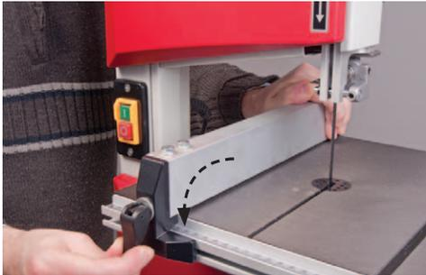
**Step 4** Locate the angled bolt (K), screw the threaded end of the bolt into the threaded hole to the top of the bandsaw frame and, using the supplied 10mm spanner, tighten with the nut to lock the bolt in position, see fig 09. Find the push stick (F) and hook it onto the angled bolt (K), see fig 10.
