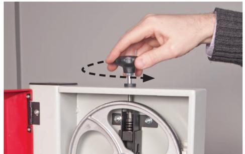
Slacken the blade by turning the tensioning wheel anti-clockwise
