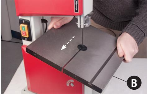
**Step 2** Place a shake proof washer (H) over each M6 bolt (G), screw the bolts through the tilt quadrant into the table and tighten using the supplied spanner, see fig 03.
