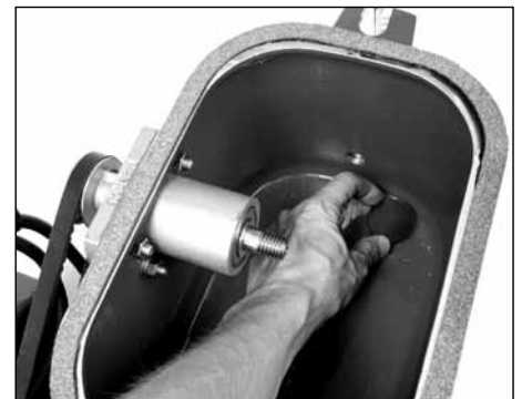
Fig. 5. Secure sludge plug
