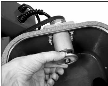
Fig. 36. Convex or recessed side of blade flange
